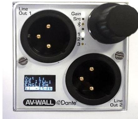
When powered, the 6 White led lights on the AV-WALL-DT4oB front face will flash and then the lights will flash alternatively until the device is switched on.
