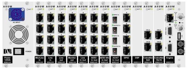
Figure 40: AXUM Digital audio system 19" Rack
