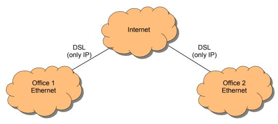
Here you see two LAN networks, both connected to internet. With correct IP-addressing Office 1 and 2 can reach each other using the IP protocol. However, there will be no interference between Office 1 and 2 on Ethernet. In fact, you have to create the same network level-structure in your studio for correct function.
