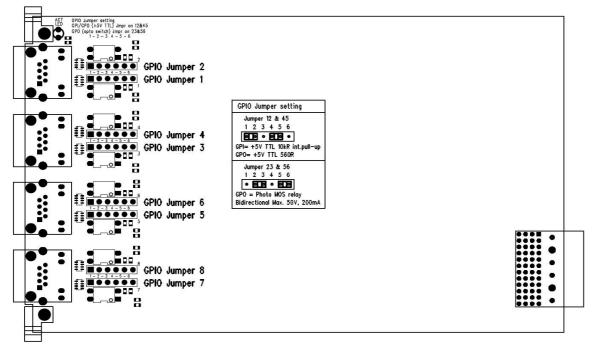
Figure 50: GPIO TTL/Relay jumper selection
