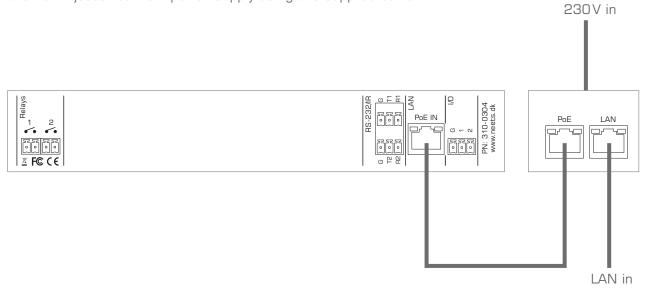
Alternatively the LiMa can be connected to a PoE enabled switch:
