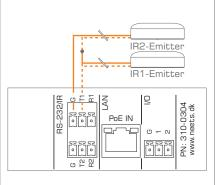
When used as RS-232 transmit port: Connect the device to T1, R1 and GND, as shown here above.
