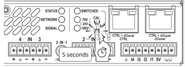
Press the mode button until it fast blinks (3 times) after 5 s, release it within 2 s after it has blinked. This will reset the amplifier to auto-IP and it will toggle the Ethernet mode and update the "Switched" indicator:
