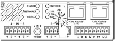
No channel will ever be assigned limiters that exceed the power of the power supply. The main reason for selecting the maximum voltage is to ensure that 25/70/100V loudspeakers will get the power selected on their tapping if a channel is using less power than it can deliver.
