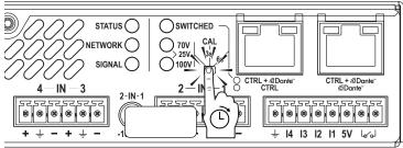
Press the mode button until it fast blinks twice after 2 s, release it within 2 s after it has blinked. This will trigger an automatic impedance measurement taking 1 s per channel. This will be made at a level that is high enough to properly measure an 8 ohm loudspeaker. If the impedance is higher the measurement might be deemed to be too noisy and it will then repeat itself automatically. Please note that it may generate an SPL exceeding 95 dB if the loudspeakers are sensitive enough.
