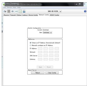
2. Use the Switch Configuration item to select the Ethernet port operation mode.
