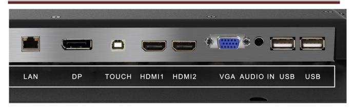
Figure 5 Rear Inputs (Bottom)
