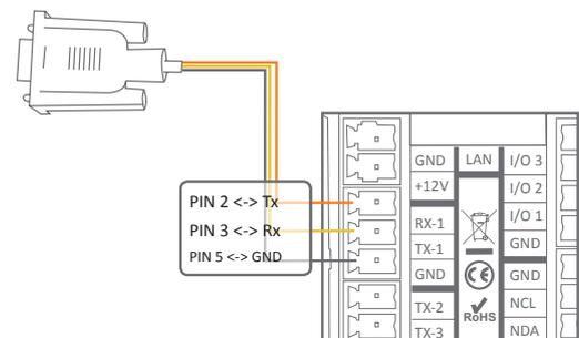
All of the RS-232/IR ports can be configured in the Neets Project Designer software either as RS-232 or as IR emitter.
