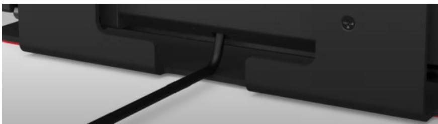
Factory reset is available via the launch button on the Parlé conferencing bars. If reset is required, push and hold the launch button for 20 seconds to reset the VBC 2500 back to its factory settings including Launch configuration.
