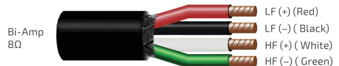
**Figure 5c.** Bi-amp wiring
